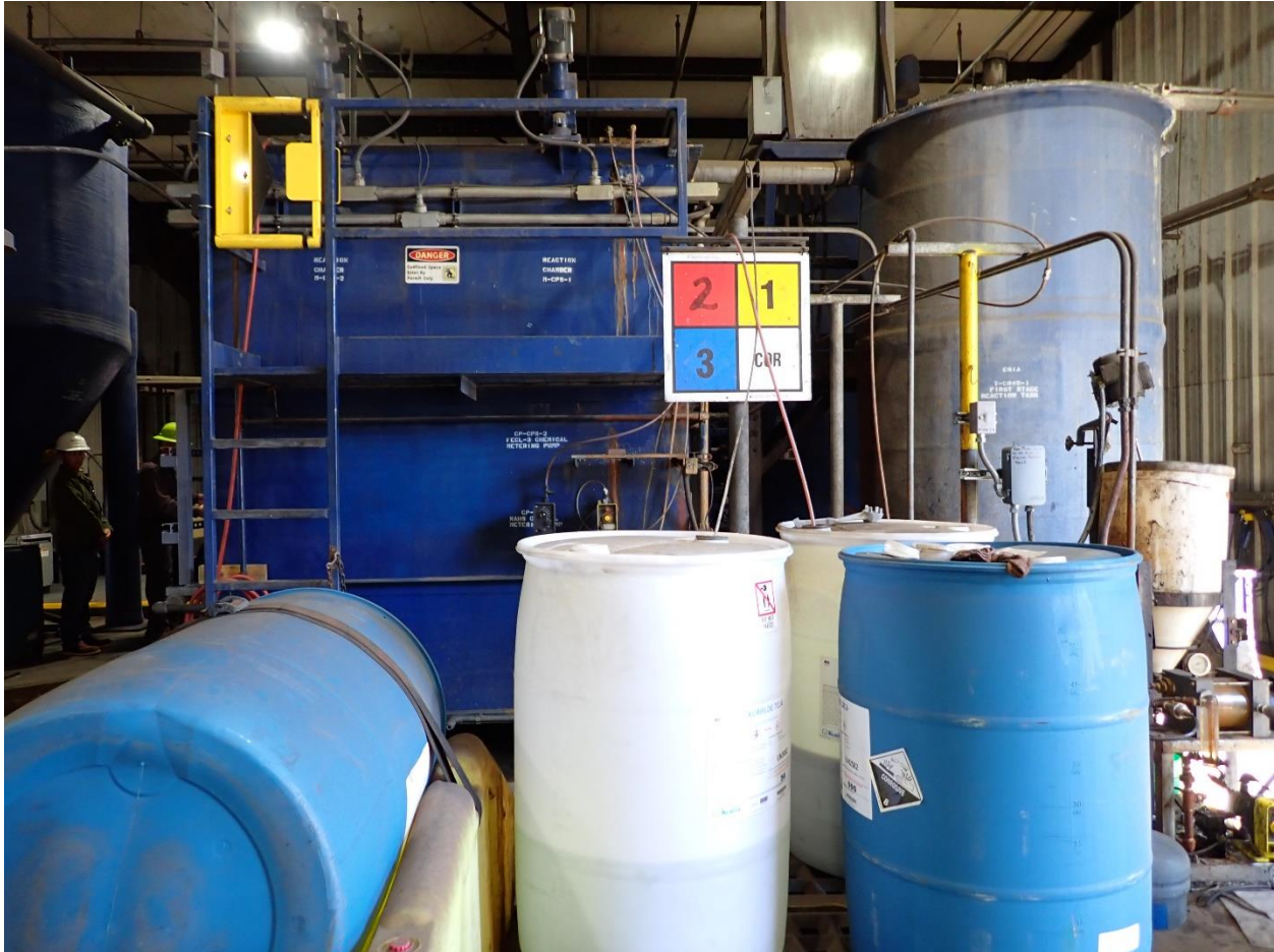
Photo 1: First stage reaction tank for pH adjustment (right of photo) and reaction chamber (left of photo)
